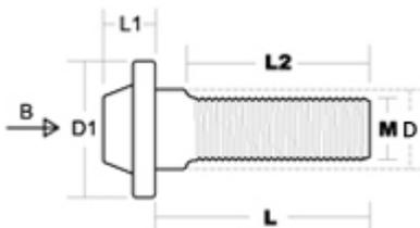
M: 10mm L: 60mm L1: 7mm L2: 33mm D1: 18mm Pas : 1.25mm D: 10mm Poids : 23g Couple de serrage : 100Nm
